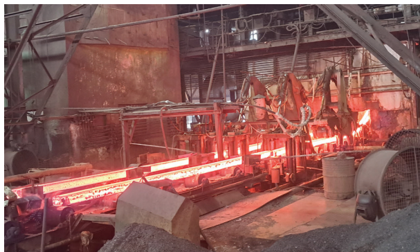
Figure 18: Continuous casting process
